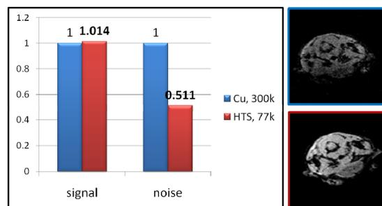
Fig. 2 Signal/noise comparison acquired by different coil settings (left). One of the images was also displayed at the right.
