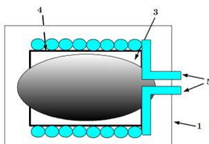
Fig. 1 (left) see-through picture of HTS volume coil, and (right) sagittal view of the coil. Each components are labeled as followed: (1) dewar (2)pick up coil (3)mice (4)HTS saddle coil (5) LN2 intake & exit.
