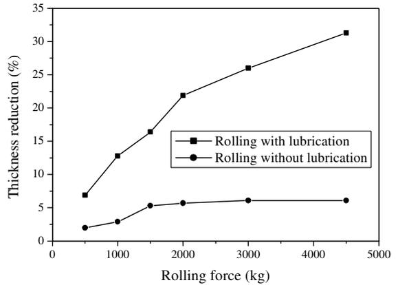
Fig. 2. Effect of lubrication on intermediate rolling reduction.
