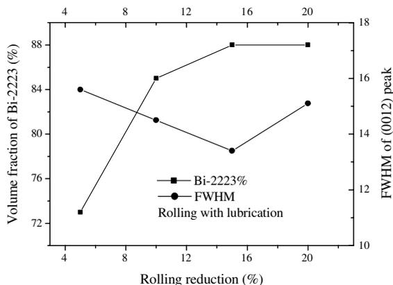
Fig. 4. The Bi-2223 phase volume fraction and degree of texturing after final heat treatment tapes rolled with different rolls.
