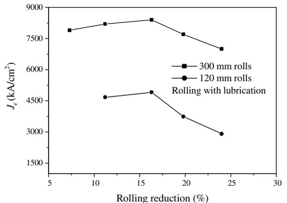
Fig. 3. Final engineering critical current density as a function of intermediate rolling reduction for tapes rolled with different rolls.
