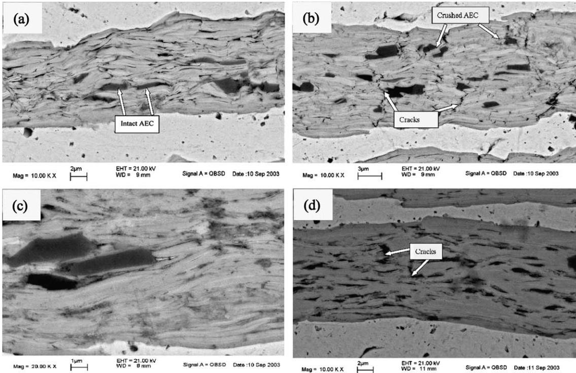
Fig. 5. Backscattered electron micrographs of (a) as intermediate rolled tape with 5% reduction, (b) as intermediate rolled tape with 20% reduction, (c) a tape with 5% IR reduction, after the final heat treatment, and (d) a tape with 20% IR reduction, after the final heat treatment.
