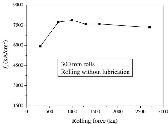
Fig. 1. Engineering critical current density versus intermediate rolling force with 300 mm rolls.
