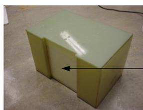
Phantom placed against the wall where the film coil is placed behind. (Coil-to-sample separation is 2 cm.)
