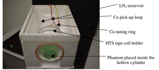
**Figure 1.** Styrofoam cryostat with a coil holder, tuning ring and pick-up loop.
