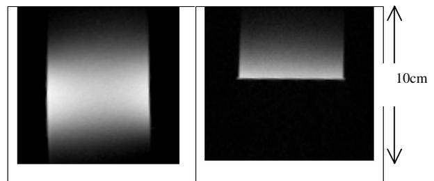
**Figure 5.** Phantom image comparison of the HTS tape coil (left) and YBCO thin film surface coil (right).
