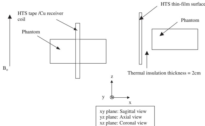
**Figure 4.** The coil and sample position inside the 0.21 T system (the cryostat is shown in this diagram).
