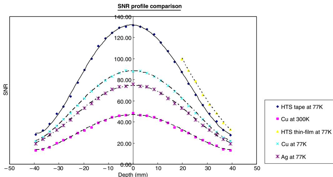
**Figure 6.** SNR profile comparison of HTS tape, copper coil, silver coil and HTS thin film surface coil.
