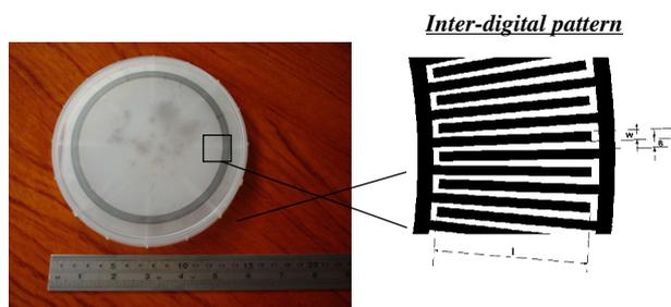
**Figure 2.** HTS thin film surface coil made of six-inch YBCO thin film. The mean diameter of the coil pattern is 5.5''.
