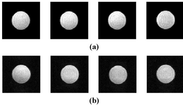
Fig. 3. Images of phantoms with conductivity of 0 S/m, 0.5 S/m, 0.9 S/m, and 1.41 S/m respectively from left to right with. (a) Superconducting receiving coil; (b) copper receiving coil of the same diameter at 77.4 K.
