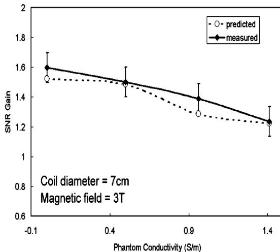
Fig. 4. The SNR gain of the HTS coil over the copper coil at 77.4 K for phantoms with different conductivities.
