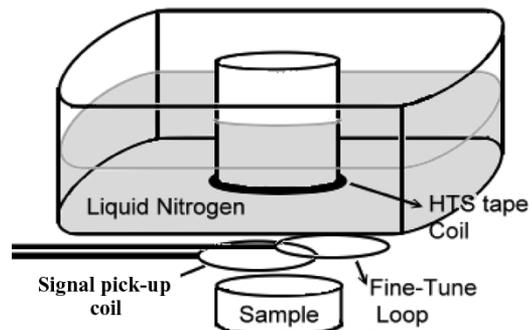
Fig. 1. Configuration of the signal pick-up coil, fine-tune loop coil and the superconducting tape coil with high Q capacitor connected in series in the imaging system.
