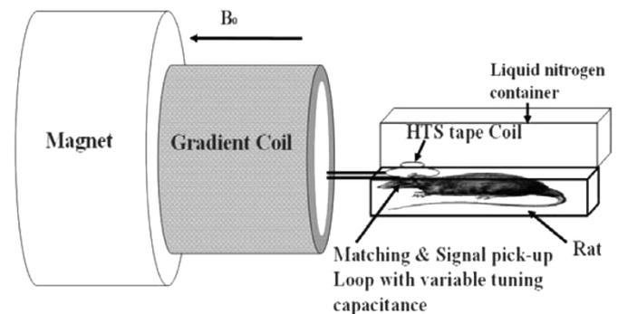
Fig. 6. Configuration of the imaging system for rats with HTS tape coil of 4 cm in diameter at 77.4 K.
