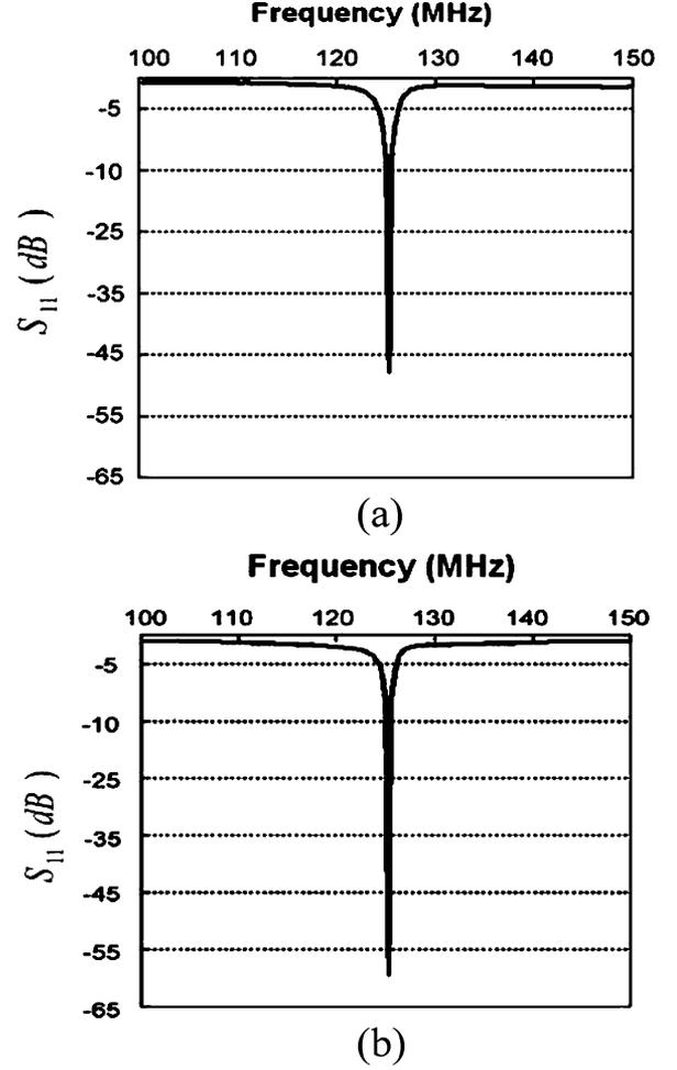
Fig. 2. The  $S_{11}$  parameter as a function of the frequency for the HTS coils with diameters of (a) 7 cm; of (b) 12 cm coupled to the tuning coil.
