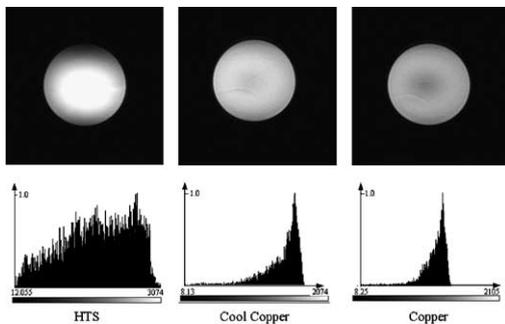
Fig. 3. Coronal phantom images and intensity histogram comparison by GE spin-echo sequence, TR = 120ms, TE = 3.4ms, NEX = 1. Field of view, the slice thickness and acquisition matrix size were  $15\text{cm} \times 15\text{cm}$ , 5mm and  $256 \times 256$ . In the histograms, the  $x$ -axis denotes intensity and  $y$ -axis denotes normalized pixel number.
