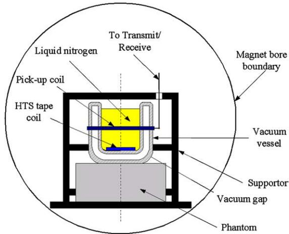
Fig. 2. Experiment setup for phantom imaging at 1.5T.
