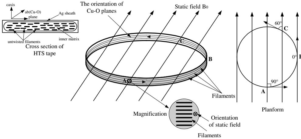
Fig. 1. The orientation of the Cu–O planes in the HTS tape filaments with respect to the static magnetic field differs with positions. For example, at points A and B, the Cu–O planes of HTS filaments are perpendicular and parallel to the static field  $B_0$  respectively. At point C, the intersection angle between filaments and  $B_0$  is  $60^\circ$ . The left section is the demonstration of the tape cross section.
