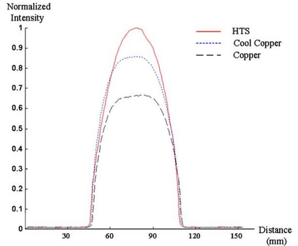
Fig. 4. Plots of intensities along the horizontal axis extracted from phantom images, in which the red, blue, black curves denote the HTS, cool copper and copper coil at room temperature, respectively.
