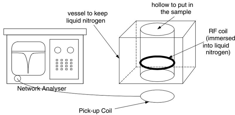
Figure 1. Experiment arrangement to measure the quality factor.
