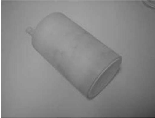
**Figure 4.** Custom-designed cryostat for housing HTS coils.
