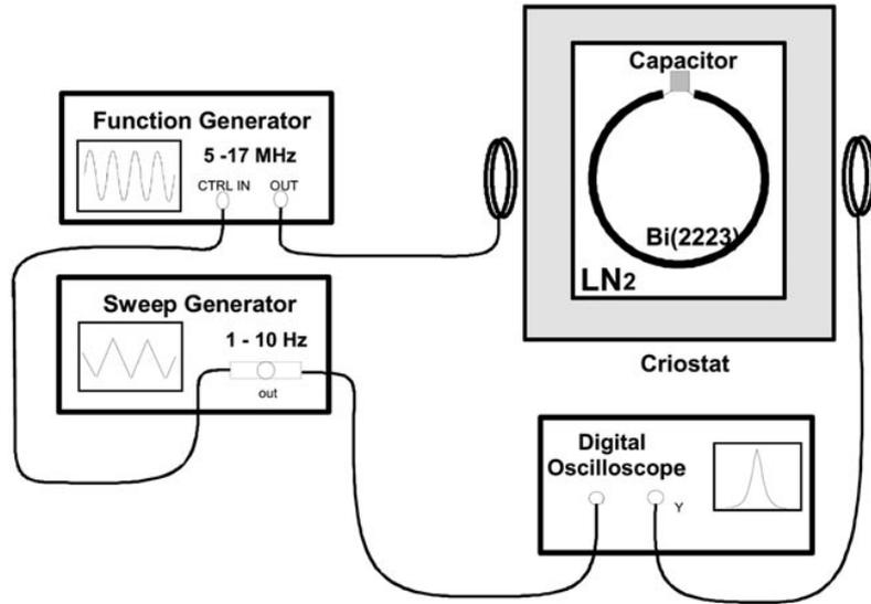
**Figure 1.** Scheme of the experimental set-up for the determination of the quality factor.
