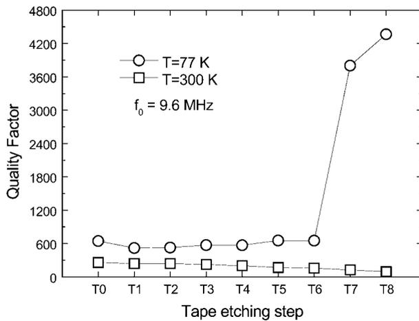
**Figure 2.** Quality factor of a single turn Bi(2223)-based L-C resonator at different stages of the etching process of the outer silver sheath (T0–T8).
